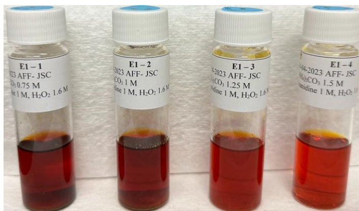
Figure 4. Solutions prepared by dissolution of \text{UO}_2 in 0.75 – 1.5 M (\text{NH}_4)_2\text{CO}_3 , 1 M [\text{C}(\text{NH}_2)_3]_2\text{CO}_3 and 1.6 M \text{H}_2\text{O}_2 [increasing in (\text{NH}_4)_2\text{CO}_3 concentration from left to right]; photographs taken at 22 h after preparation.
