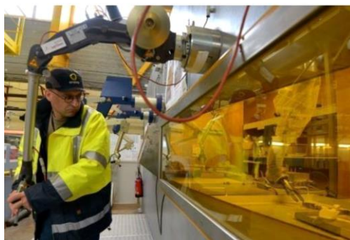
Figure 1 : Shielded enclosure with a remote manipulator
